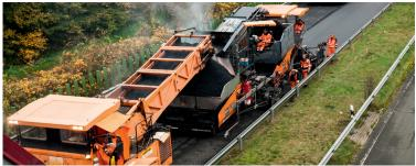
Over the past two years, the company MATTHÄI has conducted extensive experiments with asphalt screeds which are able to pre-compact asphalt courses up to 10 cm thick to a degree which approaches the results of final compaction. In collaboration with the company VÖGELE, TP 2 screeds were modified in such a way that these requirements could be met. These screeds form the basis for the development of two processes for the production of compact asphalt applying the "hot-on-hot" method.
